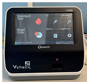
Figure 2. Immunological system Vcheck V200 (Bionote) used for the quantification of specific cardiac biomarkers, namely cardiac troponin I (cTnI) and NT-proBNP
