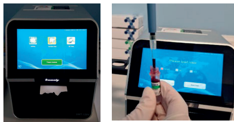
Figure 1. Biochemical lab analyzer SMT-120V. Preparing the blood for the analysis
