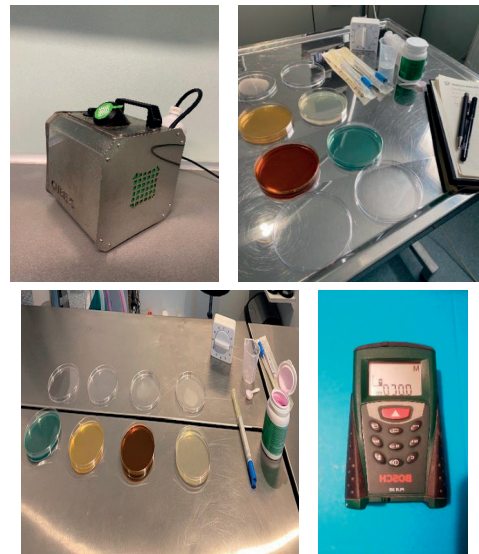
Figure 2. Materials needed: cube atomizers, Petri dishes, sterile swabs with culture medium, disinfectant solution, timer, graduated beakers, laser telemeter (Original)
