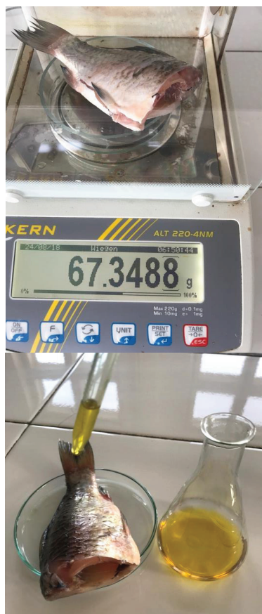
Figure 2. Carassius gibelio whole fish sample preparation: sample weighing (left); NSSO displaying onto the surface of Carassius gibelio whole fish samples in appropriate volume/weight using a micropipette (right)
