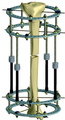
Figure 2. Full-ring circular external skeletal fixation system applied for tibia lengthening (Adapted from Zamani, A.R., Oyadij, S.O., Analytical modelling of Kirschner wired in Ilizarov circular external fixators as pretensioned slender beams, Journal of the Royal Society Interface 2009, 6:243-256)
