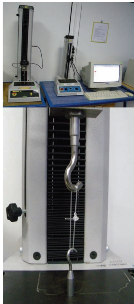
Figure 1. The servo-hydraulic materials-testing machine (MULTITEST 5-i)
